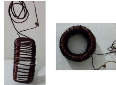
Figure 6: Picture of designed CT core and coil assembly
